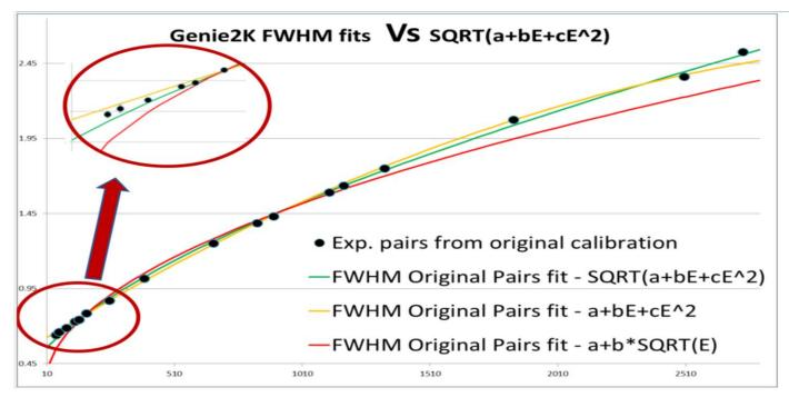
Original calibration pairs from station CALIBPHD (fresh source)
