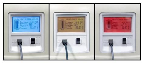
Blue LCD backlight: Unit operates normally, no action is required.
