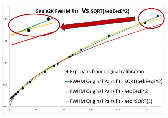
Original calibration pairs from station CALIBPHD (fresh source)
