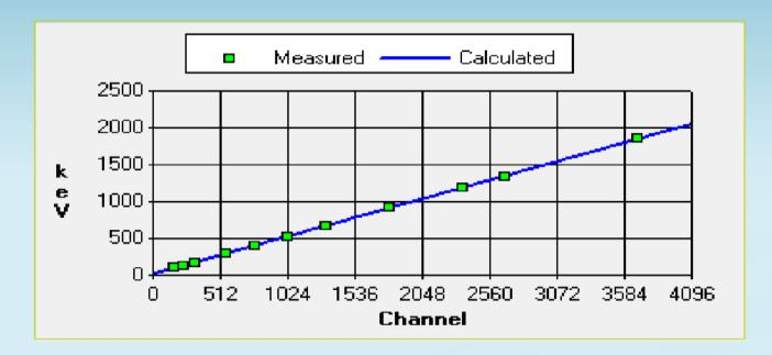
Use that calibration to assign gamma-ray energies to peaks in a spectrum, based on peak channel location
