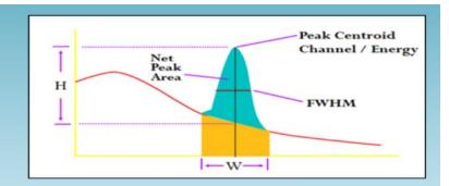
Efficiency (E) = Net counts in calibration peak at energy = E
